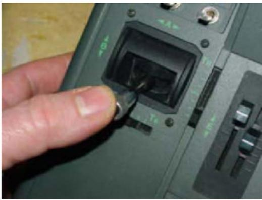
Move the trim (or switch the "engine cut" switch to on) and throttle stick back to zero and again press the right hand button (+).
