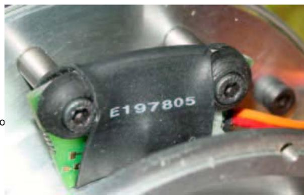
Because it receives the magnetic impulses of the rotor, it is important to assure that other electrical devices that can generate magnetic fields (e.g. servo, battery cables, pump etc), mount at least 100mm away from the engine.
