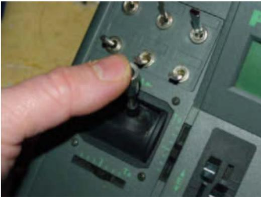
On your transmitter, raise first the trim to full and next the throttle stick to full, in this order. Ensure stick is firmly against the stop.
