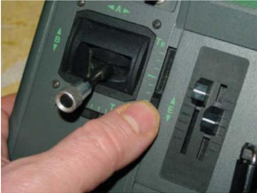
Leaving the throttle stick in the minimum position, raise the throttle trim to the full up position or switch "Engine Cut" switch to off, and again press the "+" button to store the value into the ecu.
